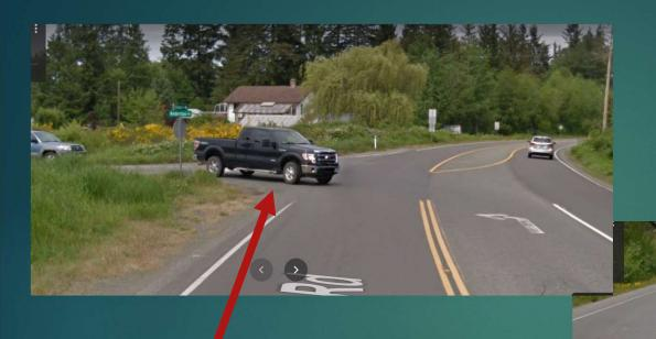
Shoulder has degraded and edges around this corner also need to be widened for safety
